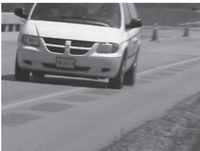
Figure 6: One of the Test Vehicles Traversing the Rectangular Rumble Strips
